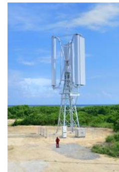
▲ Magnus x Vertical Axis Wind Turbine 10kW Prototype (Ishigaki City, Okinawa)
